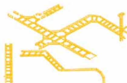
梯级式电缆桥架空间布置示意图 Spatial schematic map for ladder type cable support
